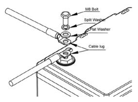
Note: Do not tighten the bolt beyond the specified torque rating of 9.5 Nm (7 lbf-ft).
