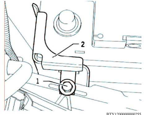
Fig. 5 Retainer bracket removal
