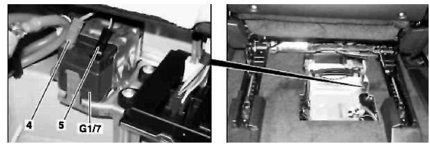
Fig. 2 Auxiliary battery removal
