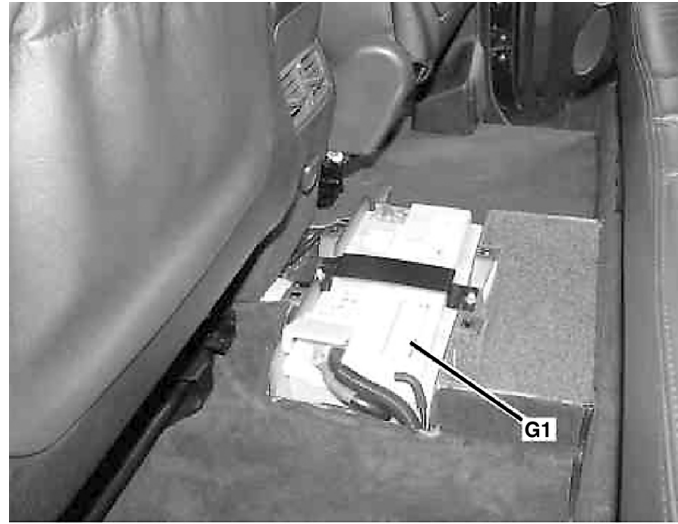
G1 On-board electrical system battery
