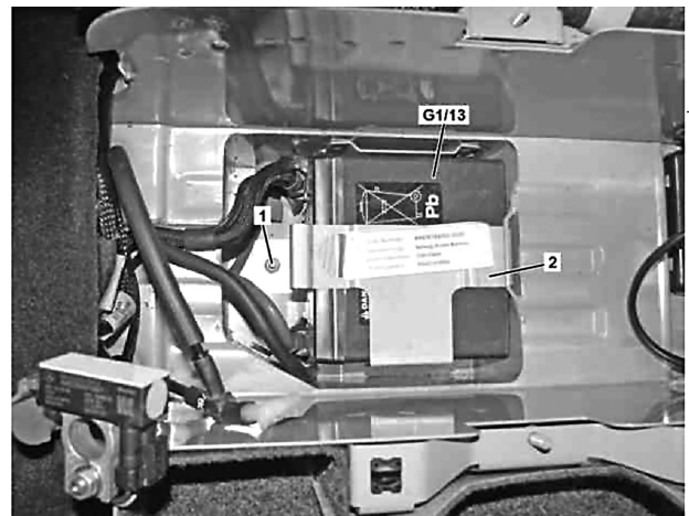
Fig. 2 Auxiliary battery removal
