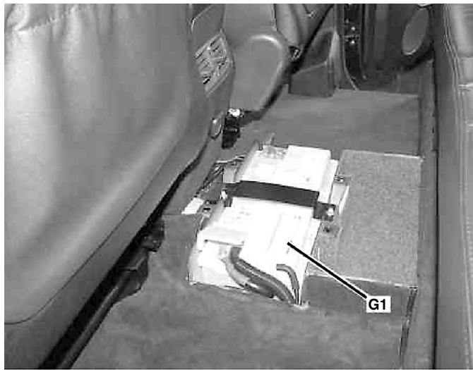
G1 On-board electrical system battery
