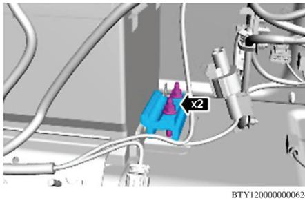
**Fig. 3 Battery hold down removal (Part 1 of 2)**
