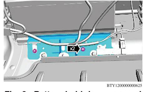
**Fig. 3 Battery hold down removal (Part 2 of 2)**
