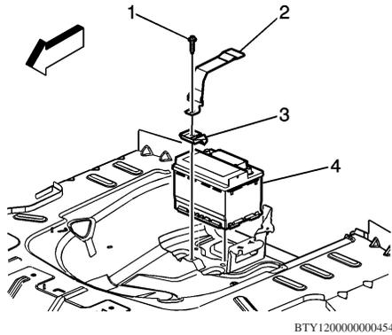
**Fig. 2 Battery removal**
