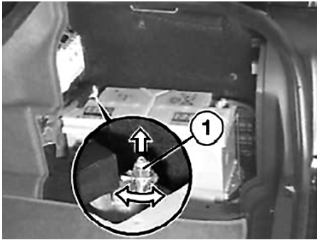
Fig. 3 Battery positive cable disconnection
