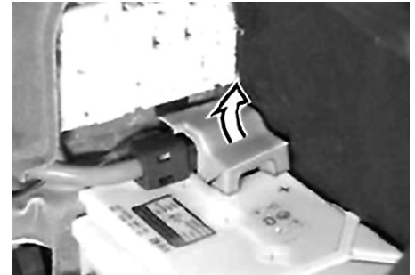
Fig. 2 Battery positive cable terminal cover removal
