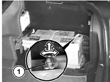
Fig. 1 Battery ground cable disconnection
