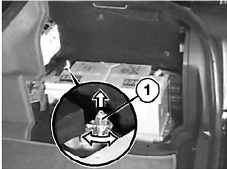
**Fig. 3 Battery positive cable disconnection**
