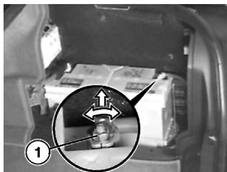
Fig. 1 Battery ground cable removal
