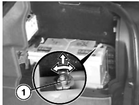
Fig. 1 Battery ground cable removal
