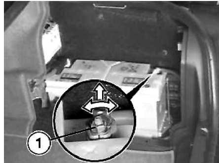
Fig. 1 Battery ground cable removal
