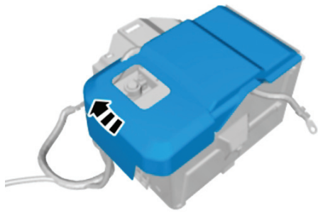
Fig. 2 Battery cover removal
