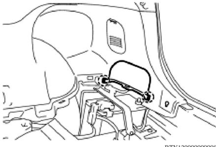
Fig. 3 No. 3 upper rear floor board plate
