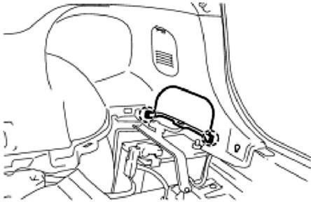
**Fig. 3 No. 3 upper rear floor board plate**
