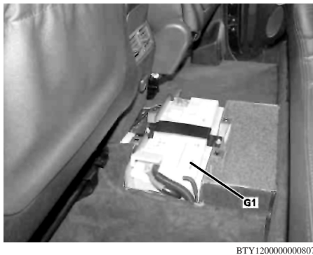
Fig. 1 Battery ground removal
