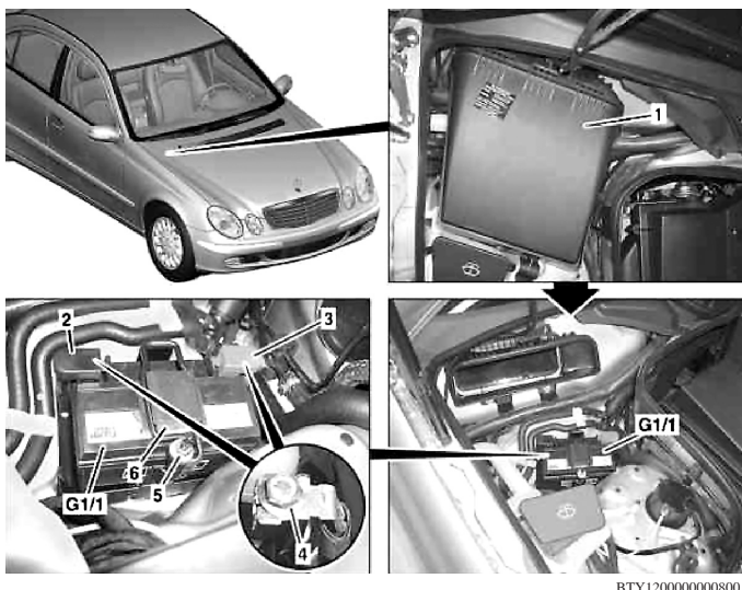
Fig. 2 Auxiliary battery removal
