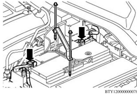
**Fig. 2 Battery removal**
