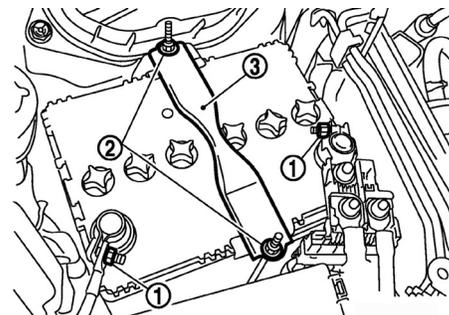
**Fig. 2 Battery fix frame removal**
